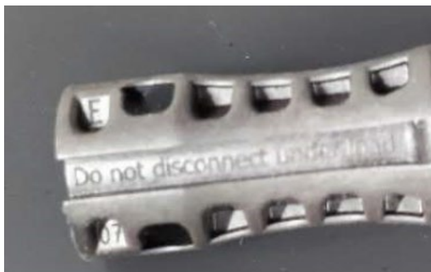
Mark (Do not disconnect under load)
